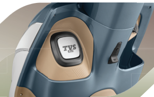
External Front Fuel Fill
